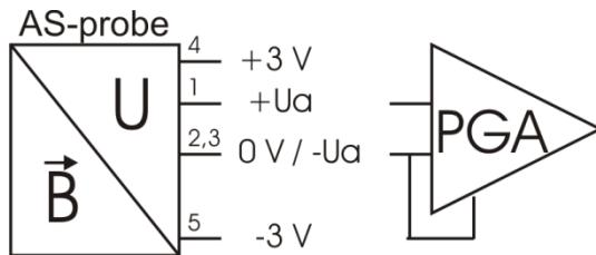
Like shown in the inner structure schematic the output signal at pin 1 is always referred to the ground signal at pin 2 and 3. This ground and the supply voltages +3 V (pin 4) and -3 V (pin 5) have to be provided from the outside.
