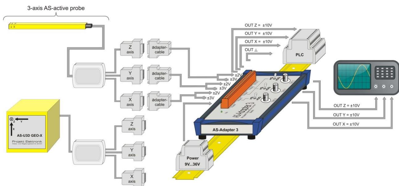
Figure 2 Connection AS-Adapter 3 with 3-axis AS-active probe
