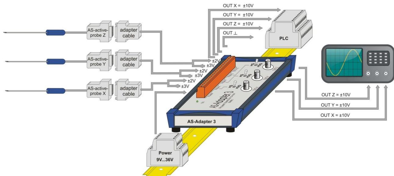
Figure 1 Connection AS-Adapter 3 with 1-axis AS-active probes
